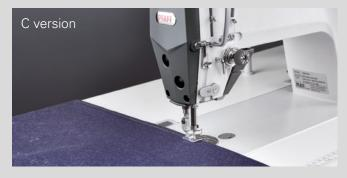
Dimmable LED light, integrated in machine head (standard on all versions)
