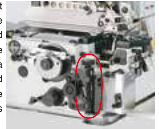
Differential-feed micro-adjustment mechanism
