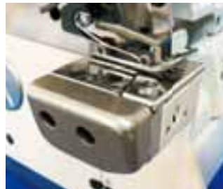
Cylinder is best-suited to runstitching and blind hemming of tubular sewing products.
